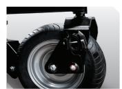
Springer Forks - Absorb bumps to provide smoother ride for operator
