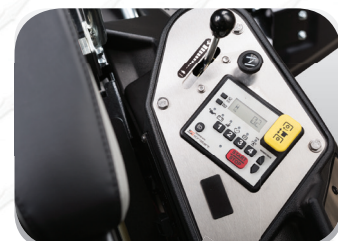
InCommand™ Console – Keyless ignition, SoftStart clutch engagement, and more
